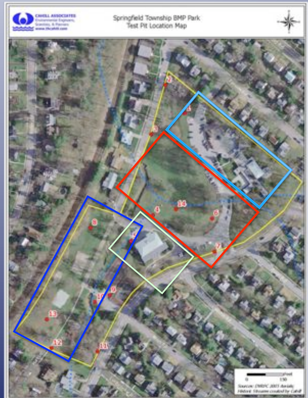
Figure 2. Approximate Test Pit (TP) Locations
